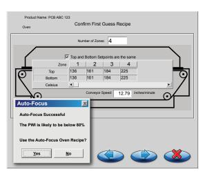
The KIC Auto-Focus and KIC Auto-Focus Power is simple, fast and easy to use, requiring minimal input or technical experience. Once the necessary criteria are provided, Auto-Focus goes to work and in seconds you are presented a suggested initial oven set up. The recipe is ranked using the Process Window Index (PWI), so you immediately know where it falls within your process specifications.
