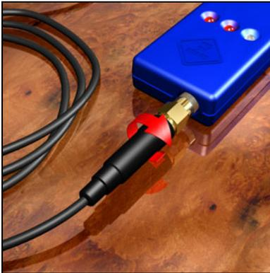
Figure 4: Connect antenna to Base Station
