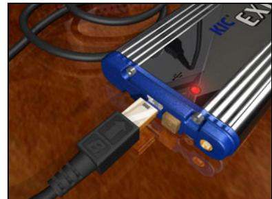
Figure 8: Connect USB cable to *KIC Explorer*
