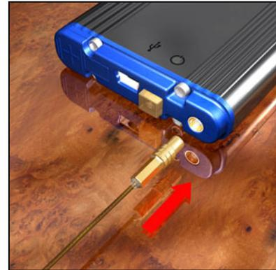
Figure 6: Connect antenna to KIC Explorer
