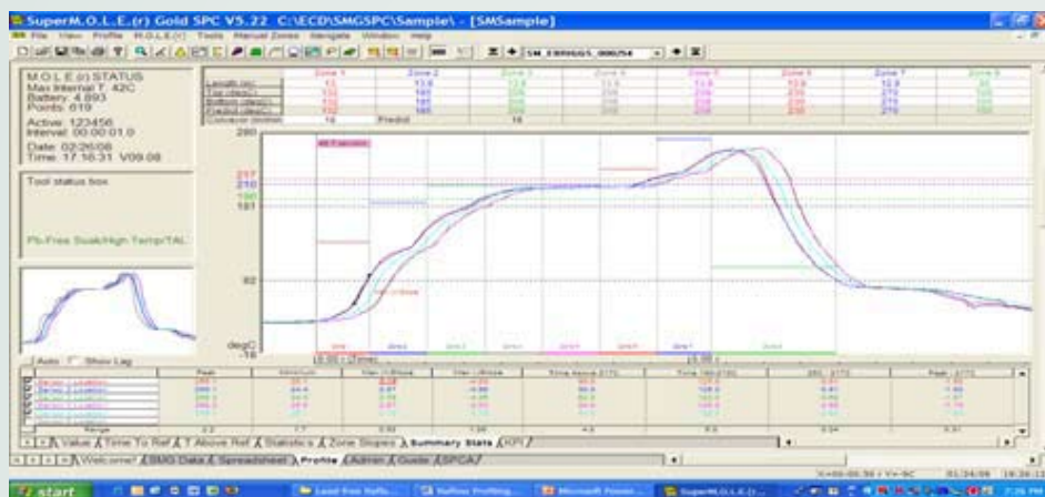
Figure 2 - Ramp/soak/spike reflow profile.
