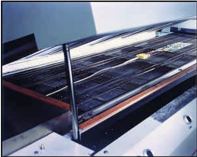
Figure 2. Computerized trailing-wire profilers consist of a single trailing cable with inputs for up to six thermocouples. To profile, the trailing cable plugs into a circuit board that is connected to the PC.
