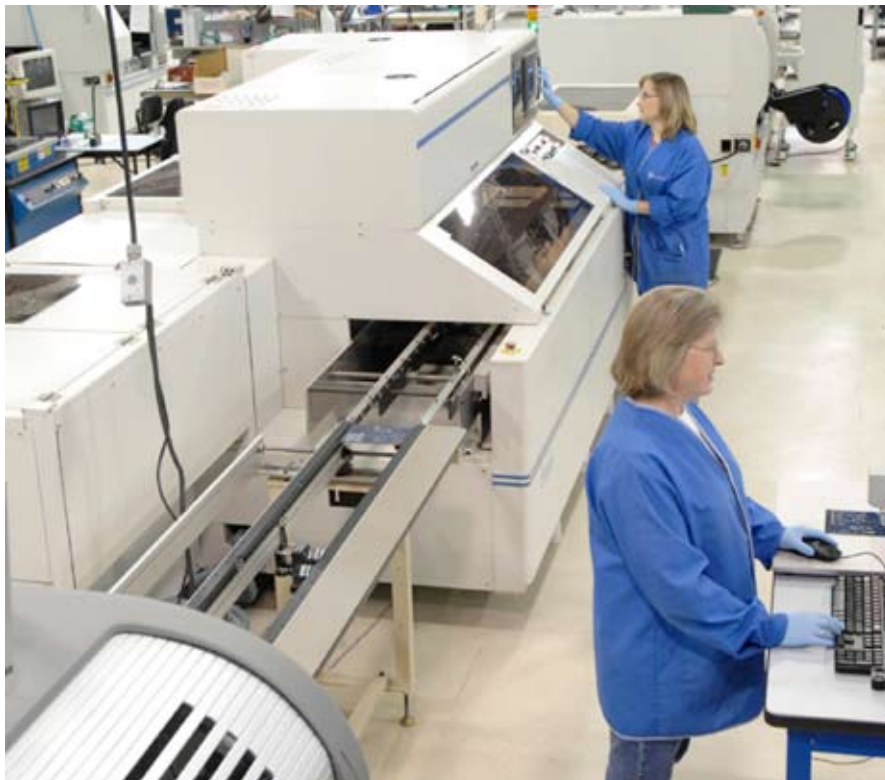
Volume component placement for LED assemblies is identical to other SMT components.
