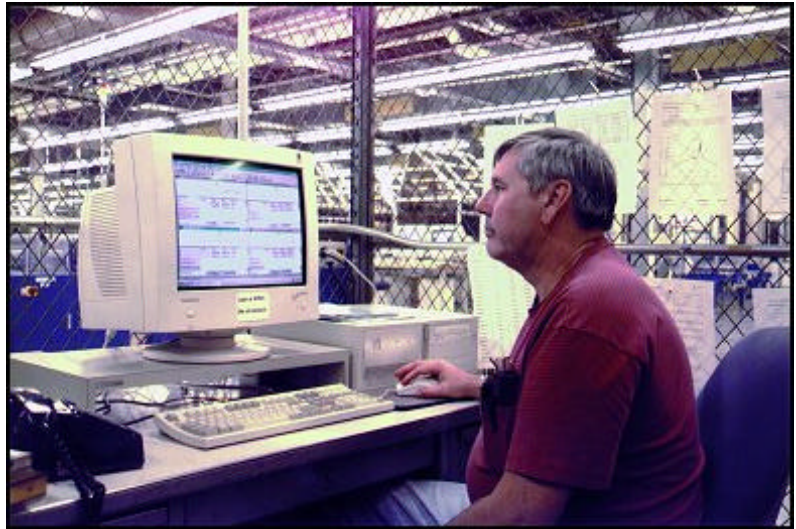
Roger Barnes, solder wave attendant at the Chrysler Huntsville assembly plant, reviews the real-time profiles for four reflow ovens simultaneously, maintaining continuous monitoring of the process and ensuring that any deviation from the pre-set parameters are identified immediately
