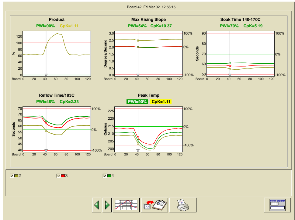
Figure 6. Statistical process control (SPC) charts with process capability (Cpk) values.
