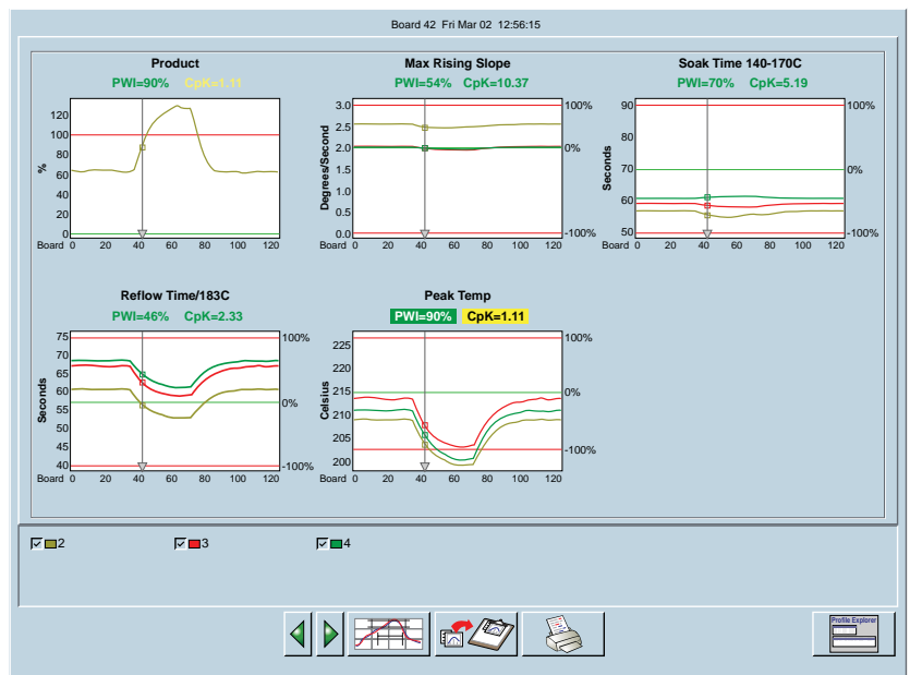
Figure 3. SPC charts. Data are plotted on real-time control charts and Cpk is calculated for such specifications as peak temperature, soak time, etc.
