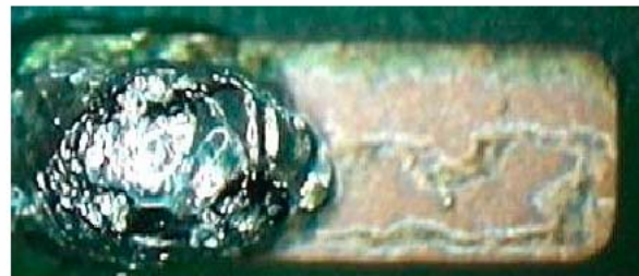
Figure 7 - Poor Wetting can be the result of exposure to high temperature for excessive time
