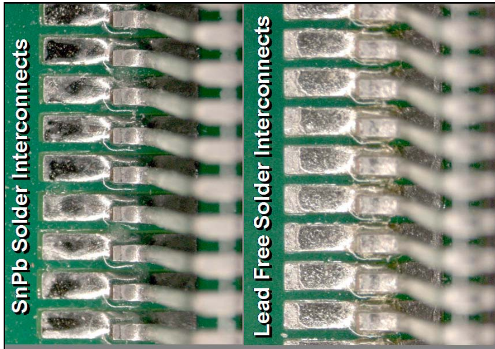
Figure 8: SnPb and SnAgCu QFP joints
