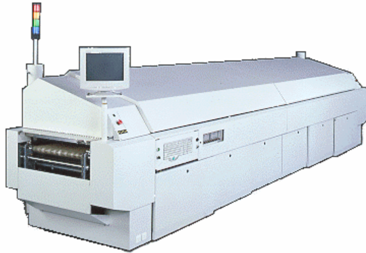
Figure 3: Typical Forced Convection Reflow Furnace
